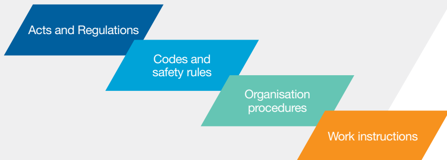
Figure 1: Hierarchy of documentation for electrical safety
